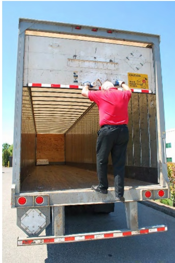
Riding the trailer door like this driver is dangerous.
