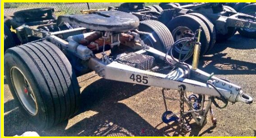
Dolly with recommended safety features: counter-balanced frame, single wide tires, drawbar-mounted oversized handles, and front leg.
