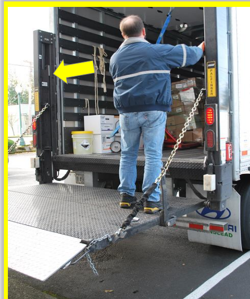
Rail-style liftgate.* Arrow points to where runner became stuck in rail.
