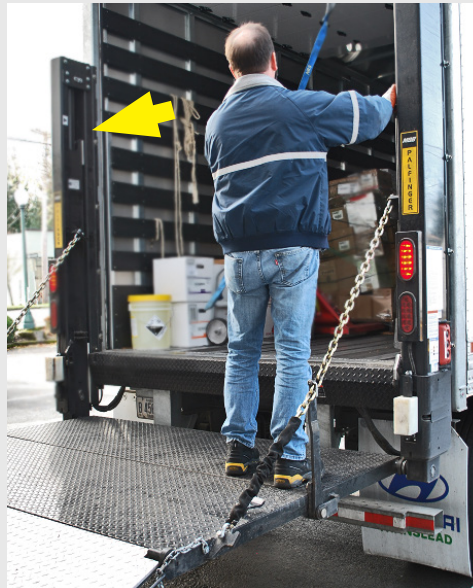
Rail-style liftgate. Arrow points to where runner became stuck in rail. Not actual liftgate in story.
