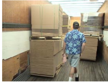
Photo 1: The top tier pallet is positioned so that the receiving customer's forklift driver can lift it off.
