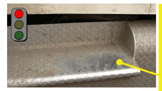
Slipping and falling from truck cab steps is a leading cause of injury for drivers.
