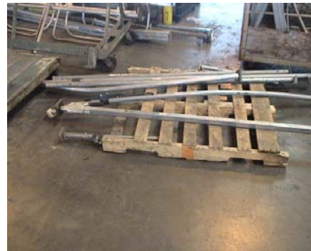
Damaged cargo bars taken out of service.
